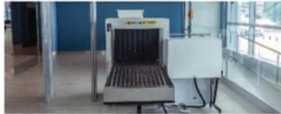
Figure 16 X-rays are useful for security scans because they have enough energy to pass through soft parts of luggage.
