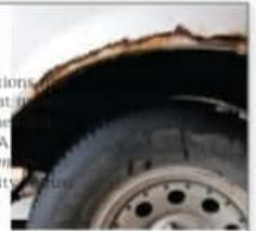
**Figure 9** This car body has rusted because of its exposure to water and oxygen. When selecting materials, it is important to evaluate the environmental conditions in which a material is going to be used.
