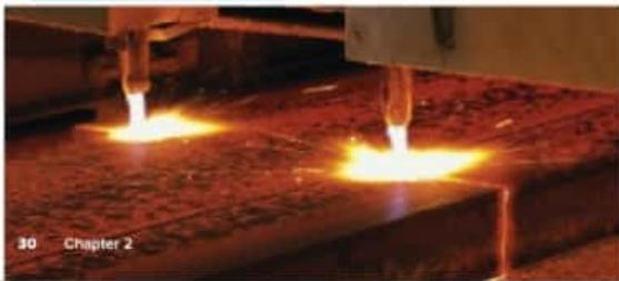
**Figure 1** This steel slab is being cut by two welding torches.
